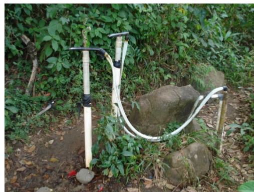
Figure 3-1: Two EMAS Flexi Pumps in a rural setting supplying overhead tanks of a household (Source: Gelhard)
