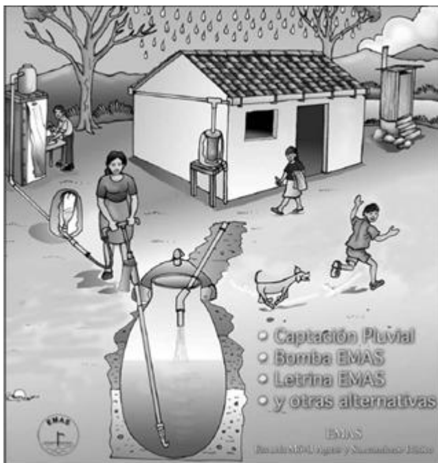
Figure 1: Promotional material for EMAS showing basic household water and sanitation technologies (Rainwater harvesting system with underground water storage tank; manual pump to lift water to small elevated tank for shower and washing clothes; ventilated latrine) (Procedamo, 2004)
